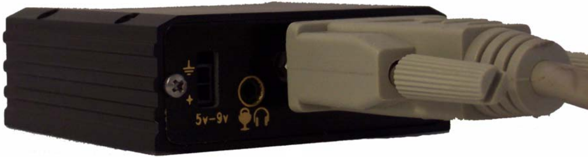
Figure 5: Connecting the Serial Cable to SA-GL
