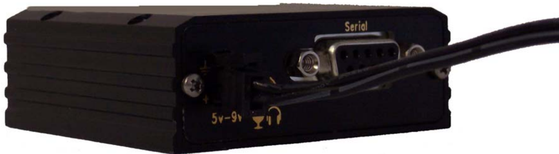
Figure 4: Connecting The Power Supply To SA GL
